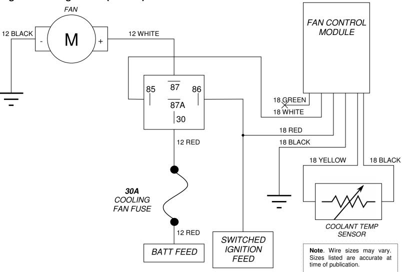
In this configuration, the one fan is run at the lower of the fan on/off points. If desired, the fan may be operated at the high fan on/off points by connecting the green wire, instead of the white wire to the relay.
