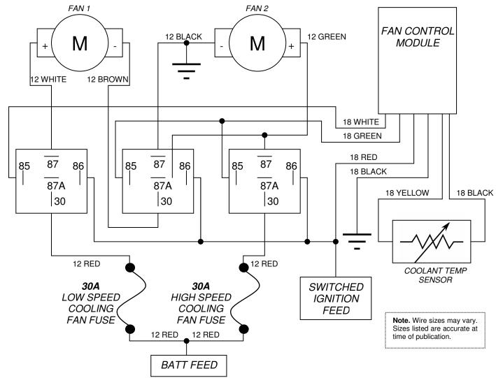
This configuration is the preferred method of fan control for systems with two radiator fans. It allows both fans to be connected in series at lower temperatures and parallel at higher temperatures. This allows the fans to run at a lower speed and consequently operate far quieter. The other benefit of this setup is that at
