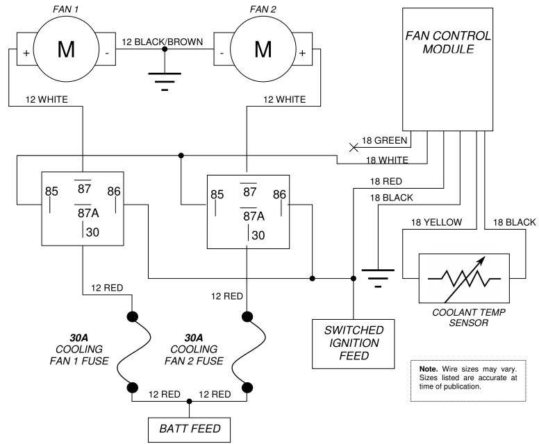
In this configuration, two fans are connected, but operate on the same control signal from the fan control module. This means they both turn on and off at the same time.
