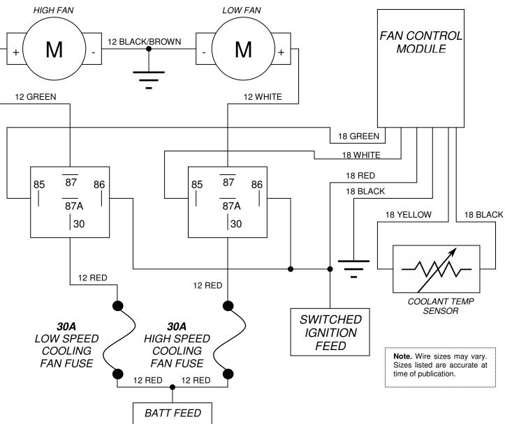
In this configuration the low fan turns on at lower temperatures, joined by the higher fan at higher engine temperatures. It is suggested that the fan shroud either have a divider between the fans, or that the fans have their own fan shrouds so that efficiency is not compromised.
