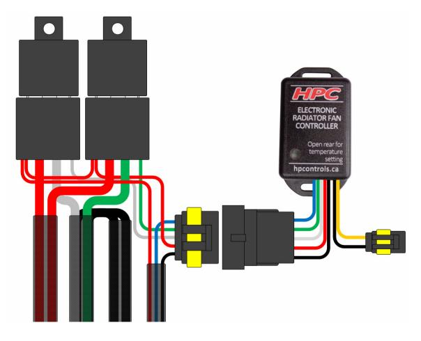
**4. Install temperature sensor wiring harness.** Plug the two pin temperature sensor harness into the temperature sensor and route it along existing wiring harnesses back to the control module. Secure the wire with supplied zip ties. If the harness is deemed too long, it may be coiled out of the way, or cut and reconnected with the two supplied pink heat shrink butt connectors.
