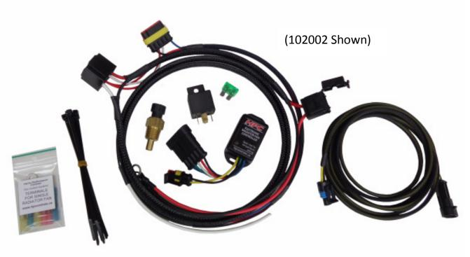
The HPC Radiator Fan Controllers provide automatic control over one or more electric radiator fan(s). These kits include a complete wiring harness for ease of installation. The module uses a temperature sensor installed in the engine to determine when to energize relays to turn on the fan(s). In addition, the module also has a remote override wire which may be connected to an existing air conditioning system or a toggle switch to turn on the fan(s).
