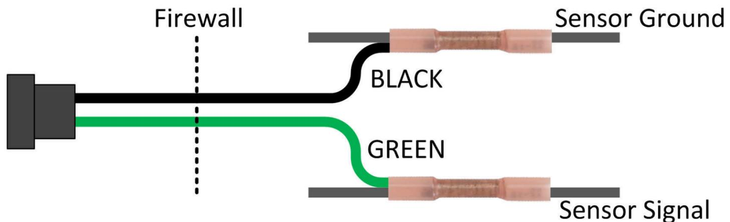
Soldering this particular connection is highly recommended. Alternatively, the installer may wish to utilize two of the provided butt connectors containing integral heat shrink tube. Ensure these two connections are water tight when complete so as to not compromise the original wiring or the sensor output.
